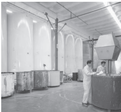
7,000-gallon resin storage and production machinery in the factory.
